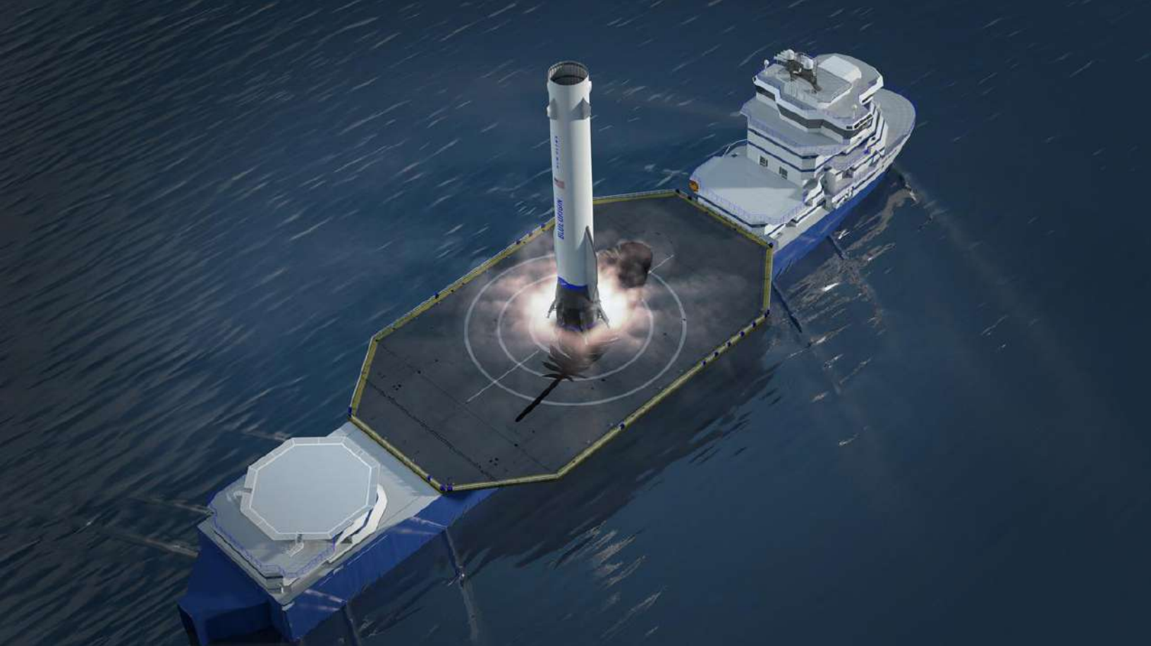
Figure 1-4: First stage landing and recovery on ocean-going platform
