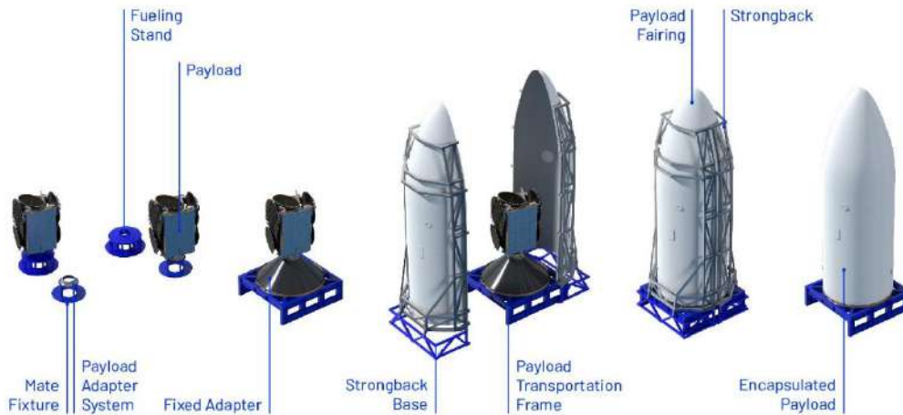
Figure 7-2: Typical payload encapsulation steps
