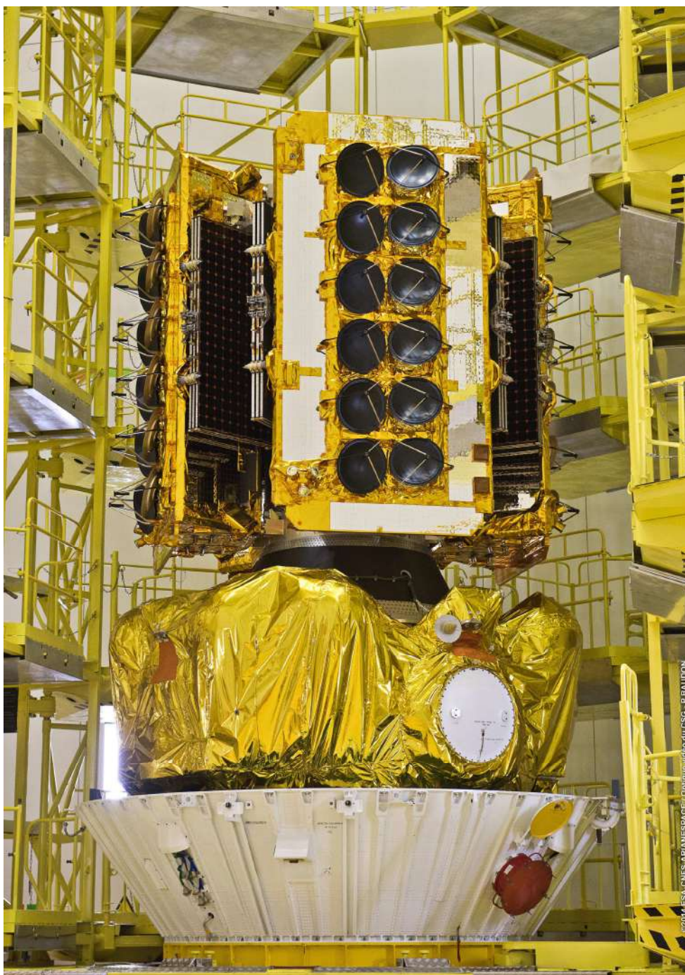
Figure A4b 3-3 Nose block with O3b dispenser ready for Fairing encapsulation
