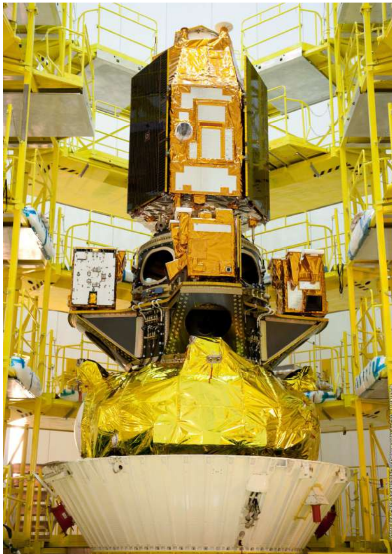
Figure A4c 1-1 Nose block with ASAP-S ready for encapsulation
