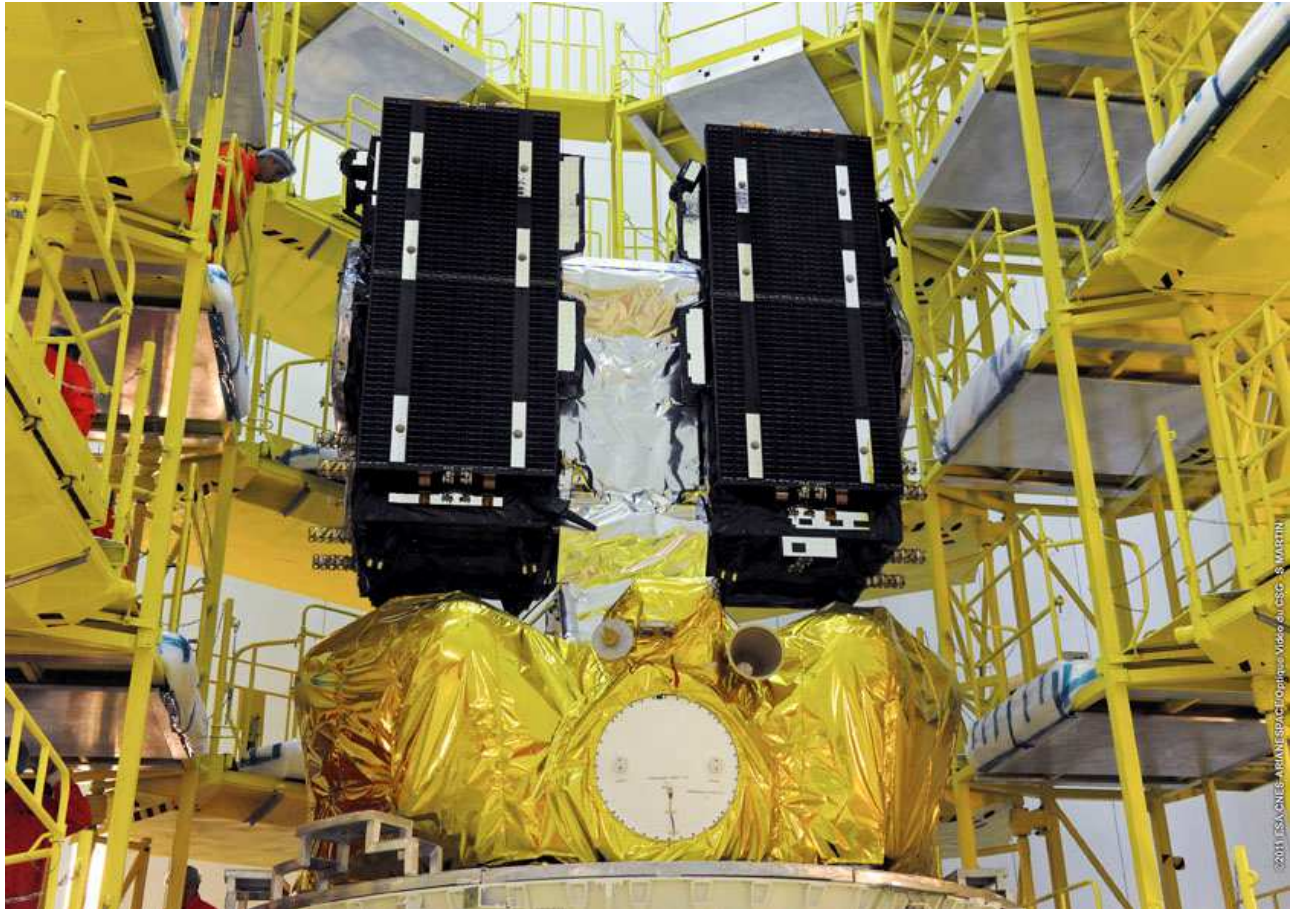
Figure A4b 2-3 Nose block with Galileo dispenser ready for Fairing encapsulation
