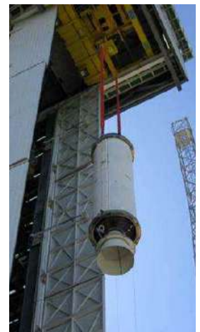
Figure 6.2.3.2.1g – Hoisting of the Z23 second stage
