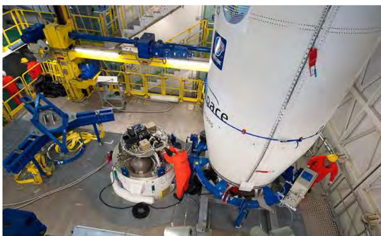
Figure 6.2.3.2.1n – PAC hoisting to the upper platform
