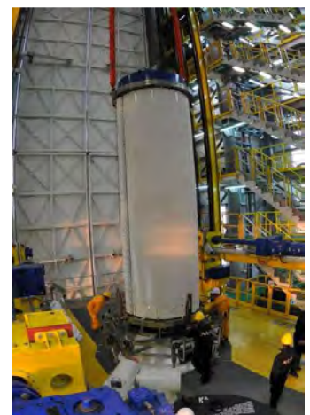
Figure 6.2.3.2.1g – Hoisting of the Z23 second stage
