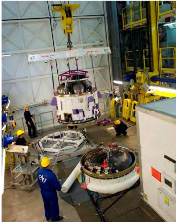
Integration of the AVUM module onto the Z9 third stage
