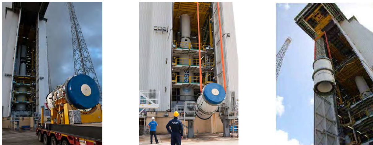
Figure 6.2.3.2.1i – Transporter arrival in front of the mobile gantry, hoisting of the Z9 third stage with the 2/3 interstage
