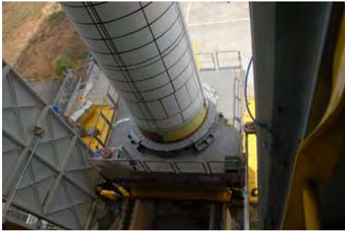
Figure 6.2.3.2.1e – Hoisting and integration of the 1/2 interstage
