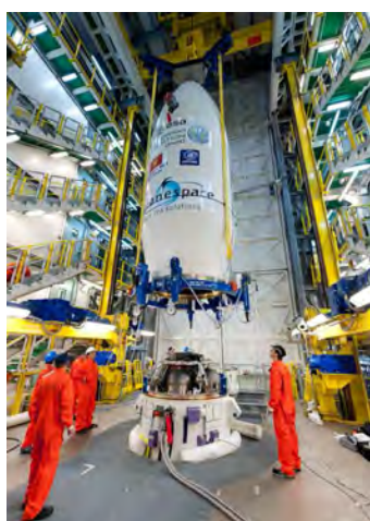
Figure 6.2.3.2.1o – PAC final positioning atop the Vega launcher inside the mobile gantry
