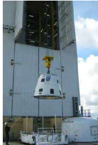
Figure 6.2.3.2.1e – Hoisting and integration of the 1/2 interstage
