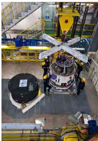
Figure 6.2.3.2.1l – Hoisting of the AVUM upper stage with the 3/AVUM interstage on top of the Z9 third stage
