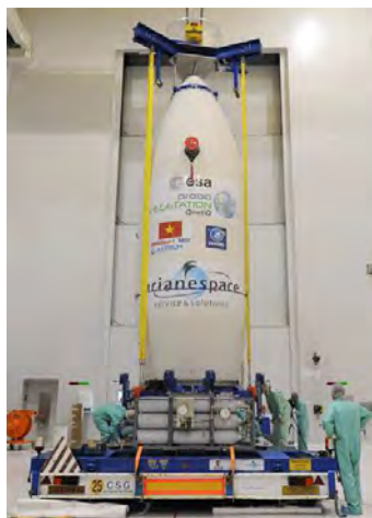
Figure 6.2.3.2.1m – After completion in the HPF building, Payload Assembly Composite (PAC) transfer to the Vega launch site
