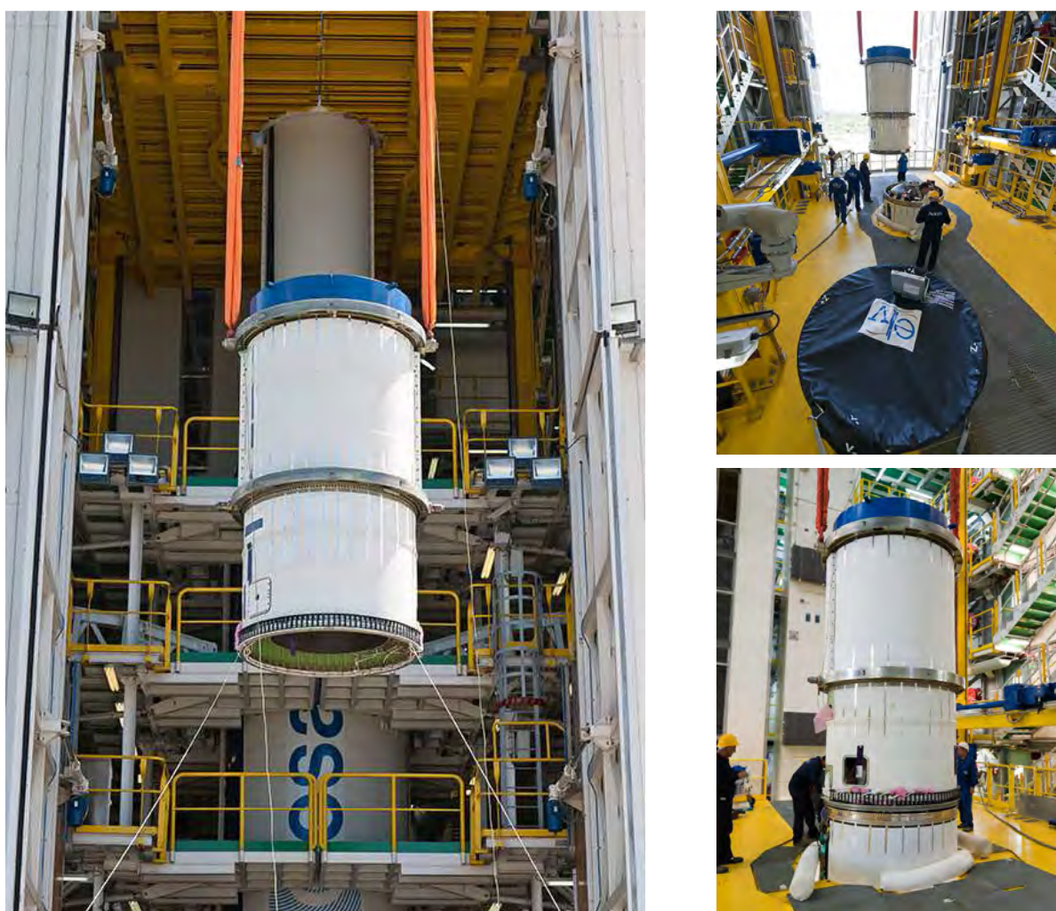
Figure 6.2.3.2.1j – Integration on the Z23 second stage, inside the mobile gantry
