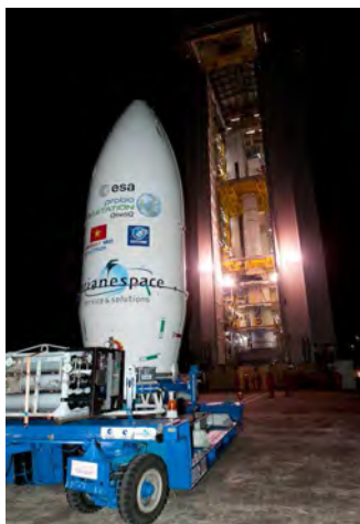
Figure 6.2.3.2.1m – After completion in the HPF building, Payload Assembly Composite (PAC) transfer to the Vega launch site
