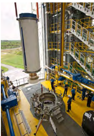
Figure 6.2.3.2.1f – Z23 second stage arrival in front of the mobile gantry
