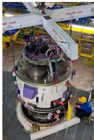
Figure 6.2.3.2.1l – Hoisting of the AVUM upper stage with the 3/AVUM interstage on top of the Z9 third stage
