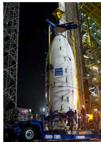
Figure 6.2.3.2.1m – After completion in the HPF building, Payload Assembly Composite (PAC) transfer to the Vega launch site
