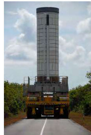
Figure 6.2.3.2.1b – Transfer to the Vega launch site by mean of a low-slung transporter vehicle
