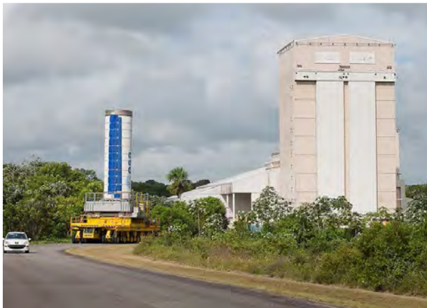
Figure 6.2.3.2.1a – Departure of the P80 first stage from the Booster Integration Facility
