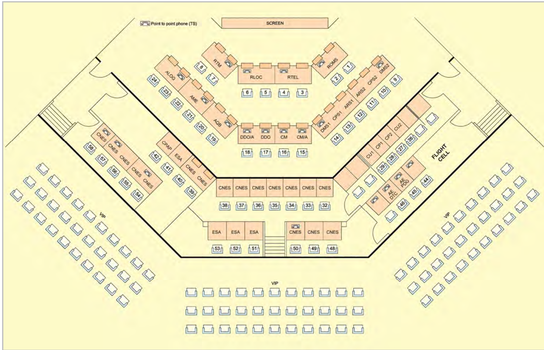
Figure 6.2.3.3b – Typical Mission Control Center (Jupiter 2) lay out
