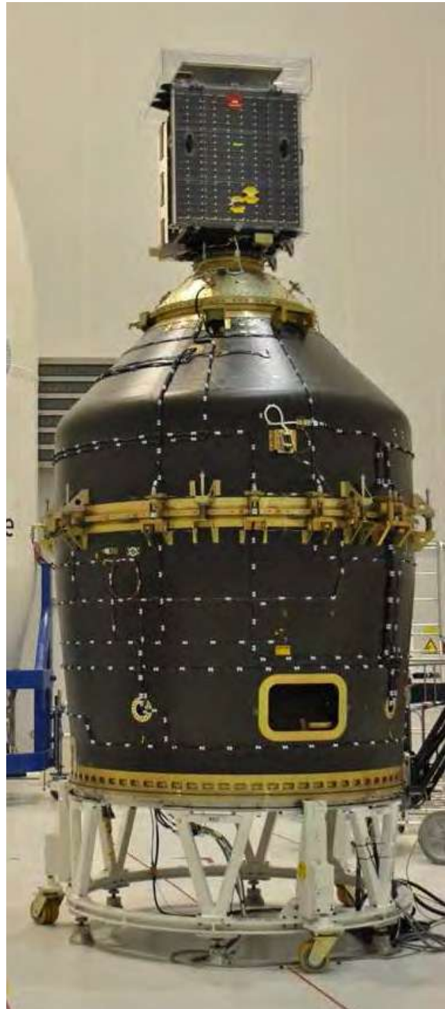
Figure A4b.1-a – Satellites integrated on the VESPA (VV02 flight)
