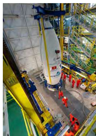
Figure 6.2.3.2.1o – PAC final positioning atop the Vega launcher inside the mobile gantry
