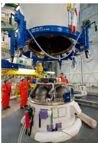
Figure 6.2.3.2.1o – PAC final positioning atop the Vega launcher inside the mobile gantry
