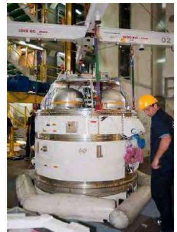
Figure 6.2.3.2.1l – Hoisting of the AVUM upper stage with the 3/AVUM interstage on top of the Z9 third stage
