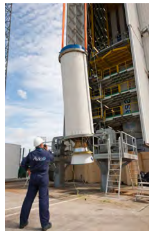
Figure 6.2.3.2.1g – Hoisting of the Z23 second stage
