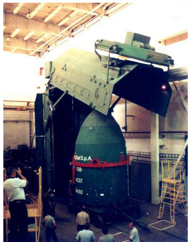
Figure 7.5-1 SHM Loading into Transporter Erector
