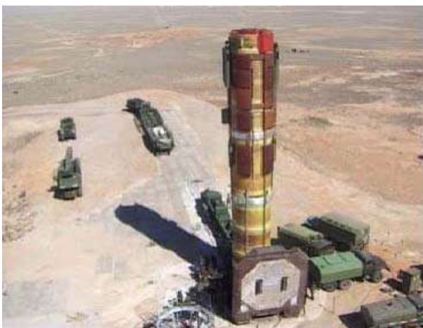
Figure 7.1-1 Loading of TLC Containing LV 1 st and 2 nd Stages into Silo Launcher
