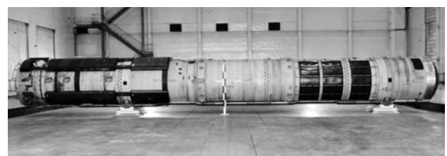
Figure 4.1-2 SS-18 1 st and 2 nd Stages Inside TLC
