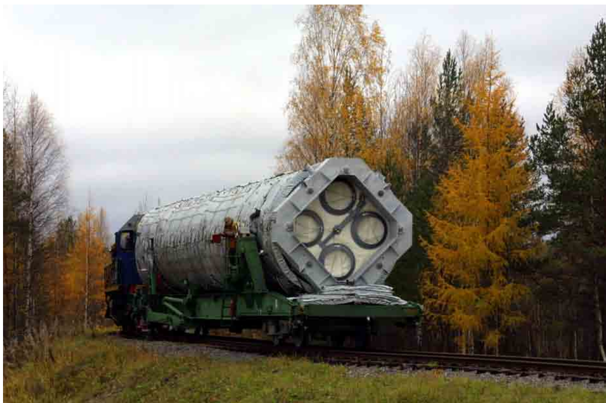
Figure 1-11 Rockot booster delivery to the launch pad.
