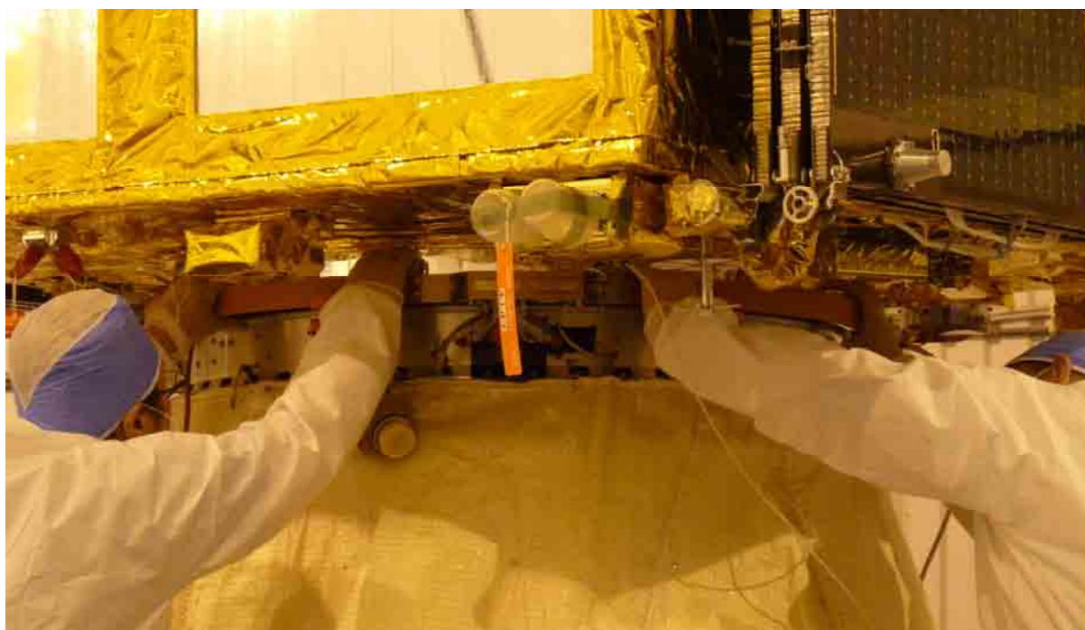
Figure 1-19 Spacecraft mating with the adapter system using an EADS CASA clamp band.
