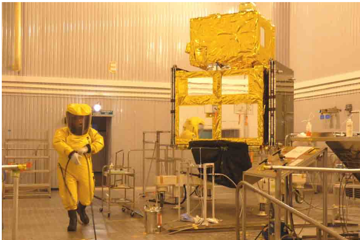
Figure 1-18 Spacecraft hydrazine fuelling on EUROCKOT fuelling platform.
