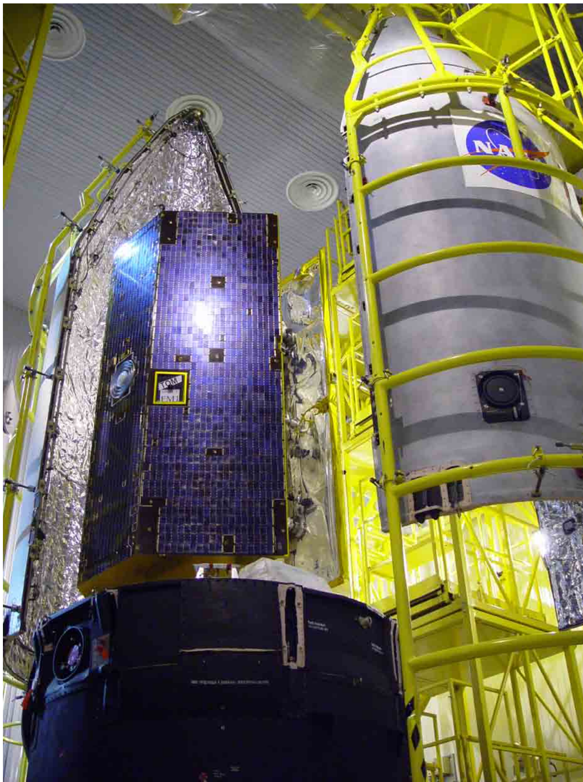
Figure 1-23 Final encapsulation operations (GRACE, 2002).
