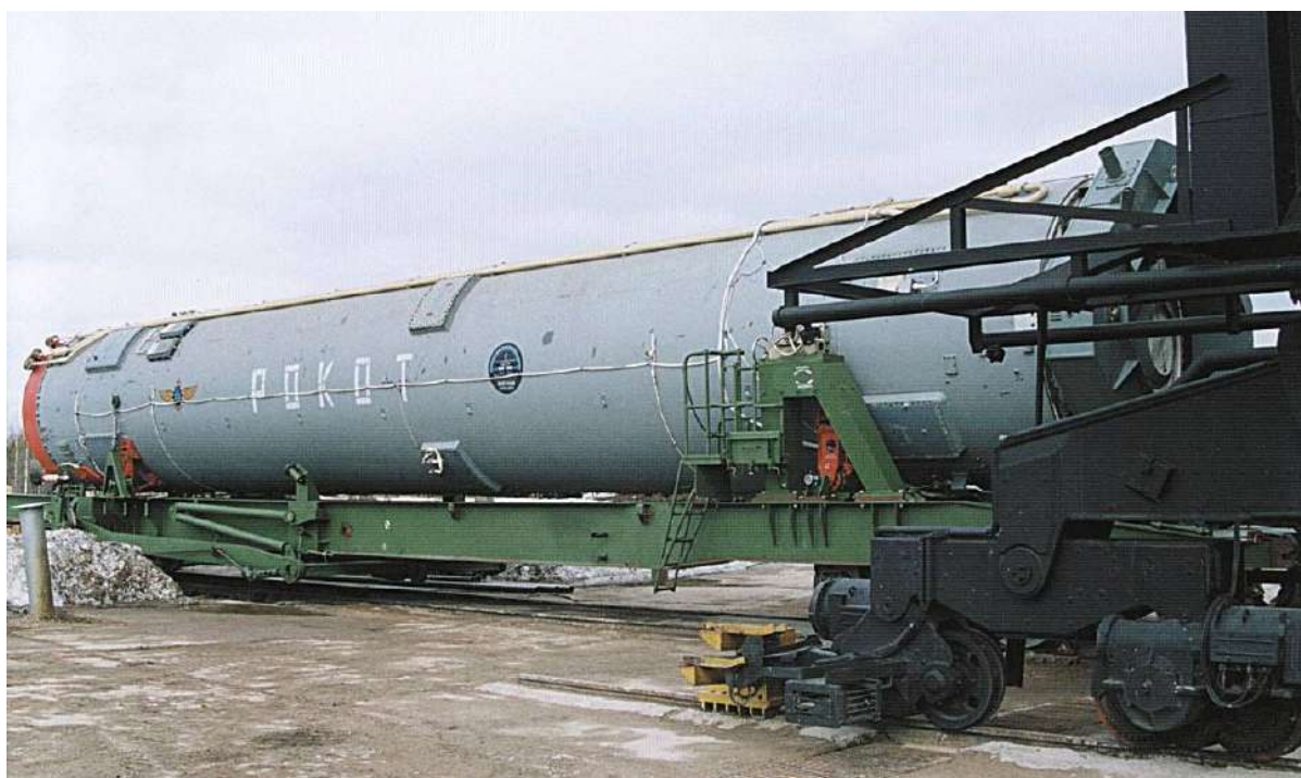
Figure 1-12 Booster installation at the launch pad.
