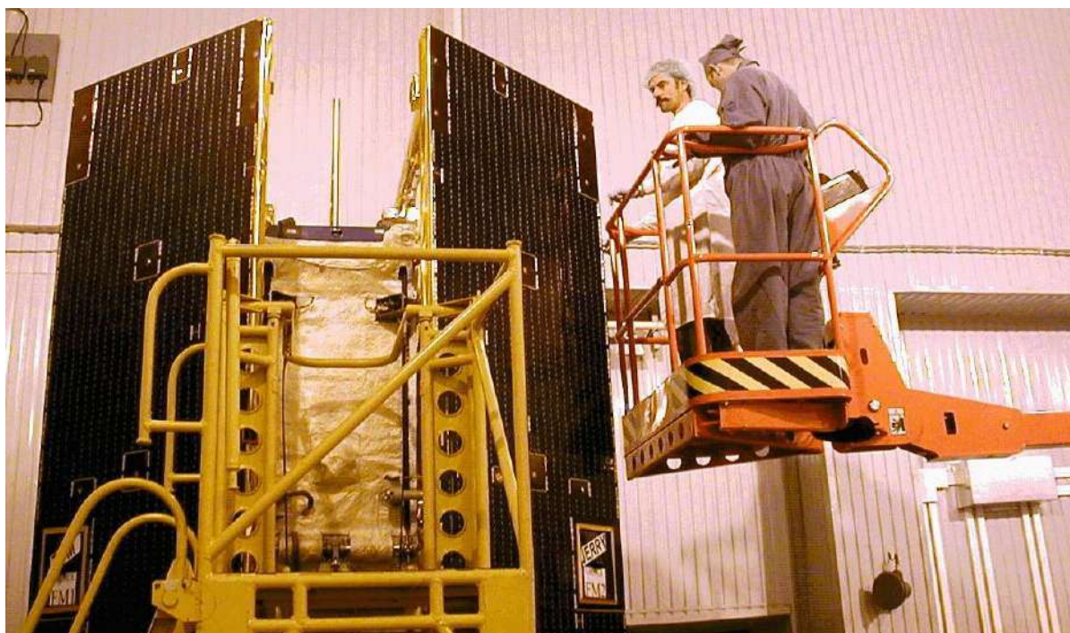
Figure 1-16 Spacecraft installation on the multi-satellite dispenser (GRACE, 2002).
