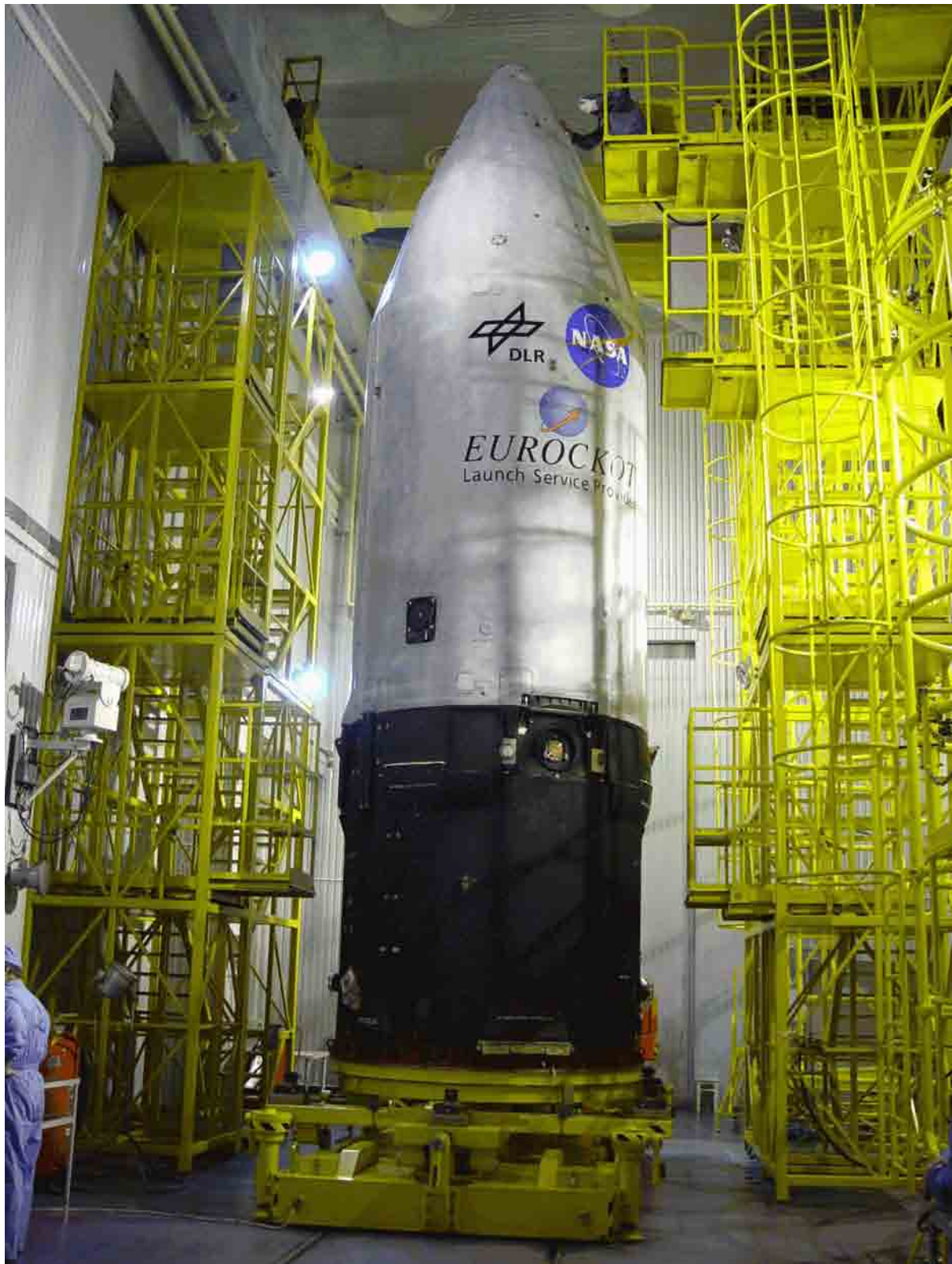
Figure 1-25 Completion of payload encapsulation (GRACE, 2002).
