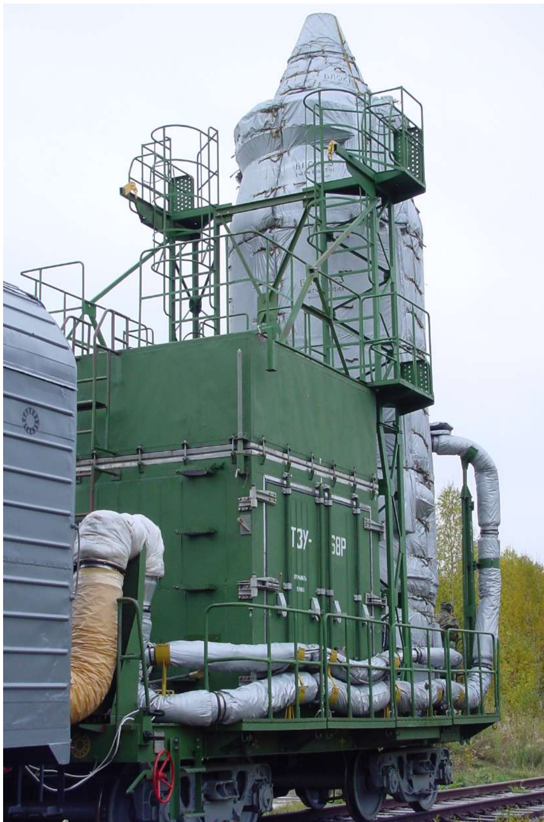
Figure 1-27 Rockot upper composite on its way to the launch pad.
