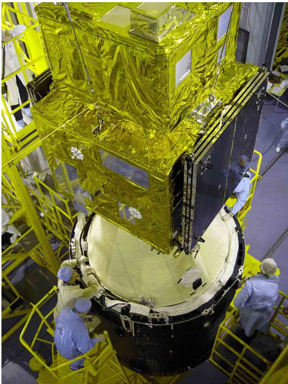
Figure 1-21 Mating with the Breeze-KM upper stage (SERVIS-1, 2003).
