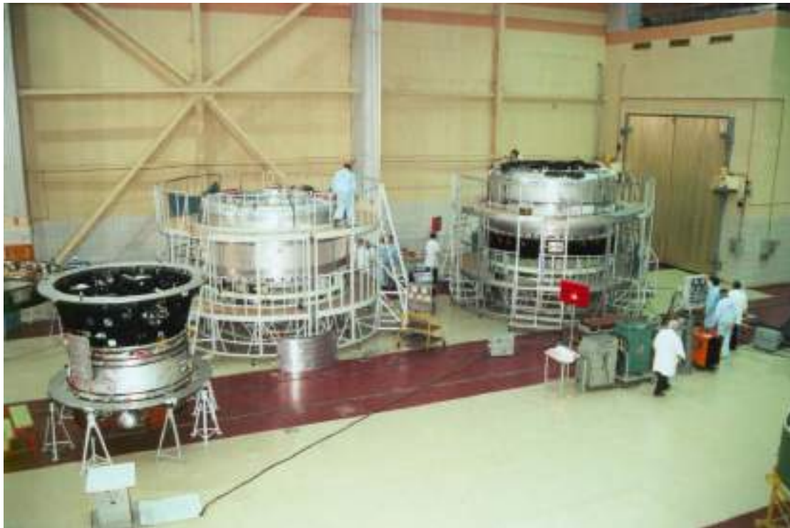
Figure 1.6.4-2: Breeze M Upper Stages in Assembly Shop
