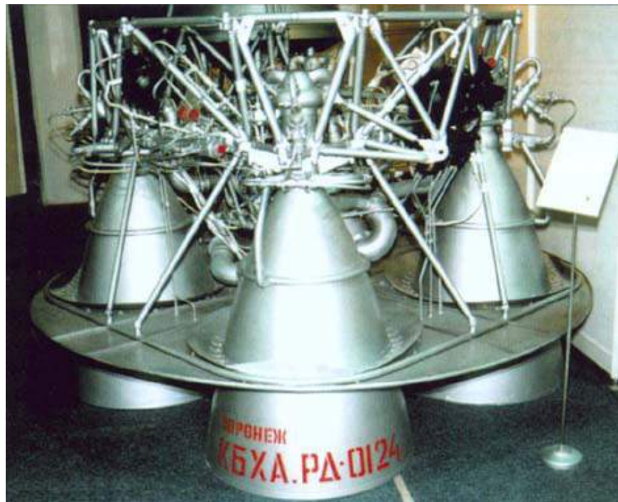
Figure 1.6.2-2: RD-0124A Liquid Propellant Rocket Engine
