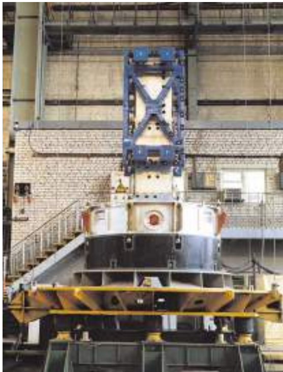
Figure 1.11-4: Upper Stage and SC Joint Vibration and Strength Tests
