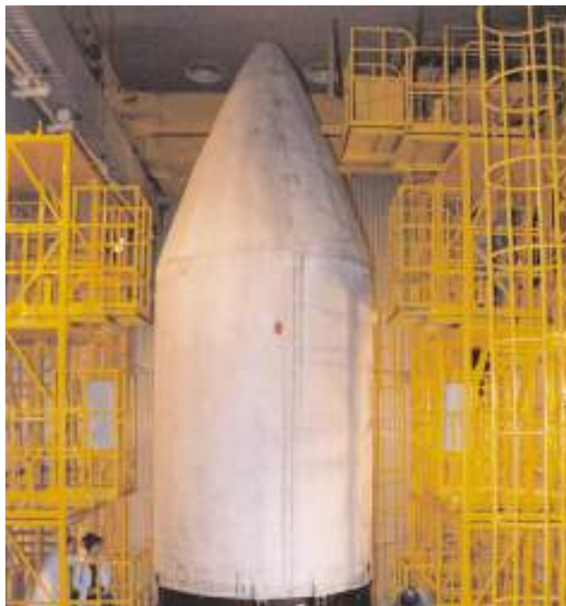
Figure 1.6.5.1-2: PLF on the Ascent Unit of the Rokot LV at the Technical Complex
