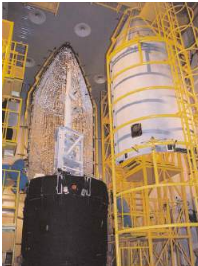
Figure 1.11-2: Assembly of Ascent Unit in Technical Complex Cleanroom
