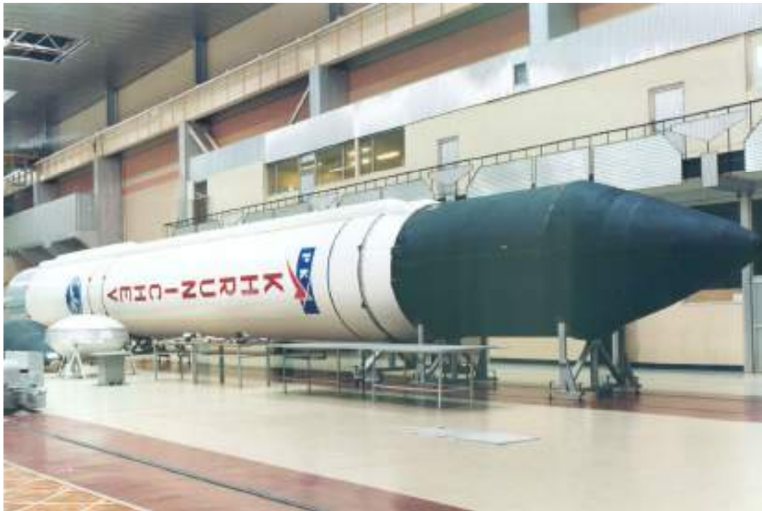
Figure 1.5.1-4: Angara 1.1 LV in Assembly Shop
