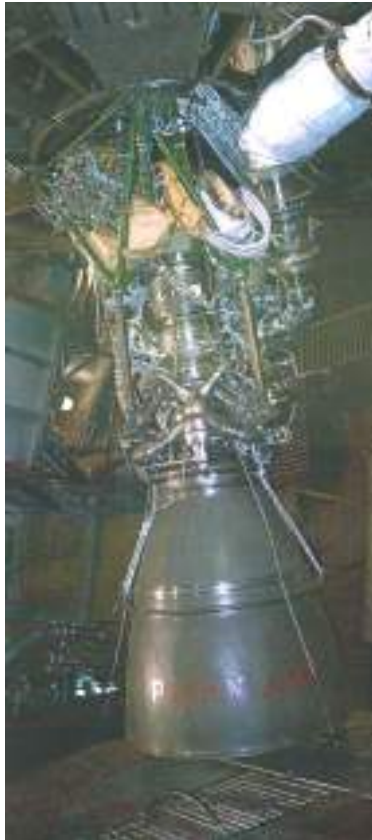
Figure 1.6.1-5: RD-191 Liquid Propellant Rocket Engine
