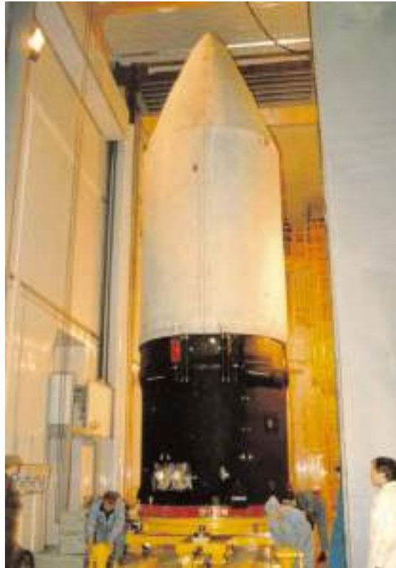
Figure 1.11-3: Transfer of Assembled Ascent Unit From Technical Complex Cleanroom
