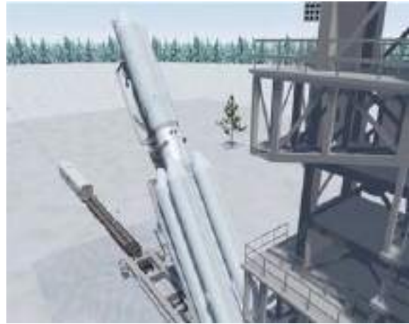
Figure 1.10.3-1: Transporting Angara A5 LV to the Universal Launch Complex and Erecting on Launch Pad
