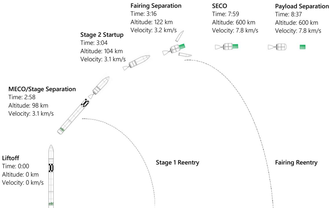
Figure 6: Reference Direct Insertion Mission Profile
