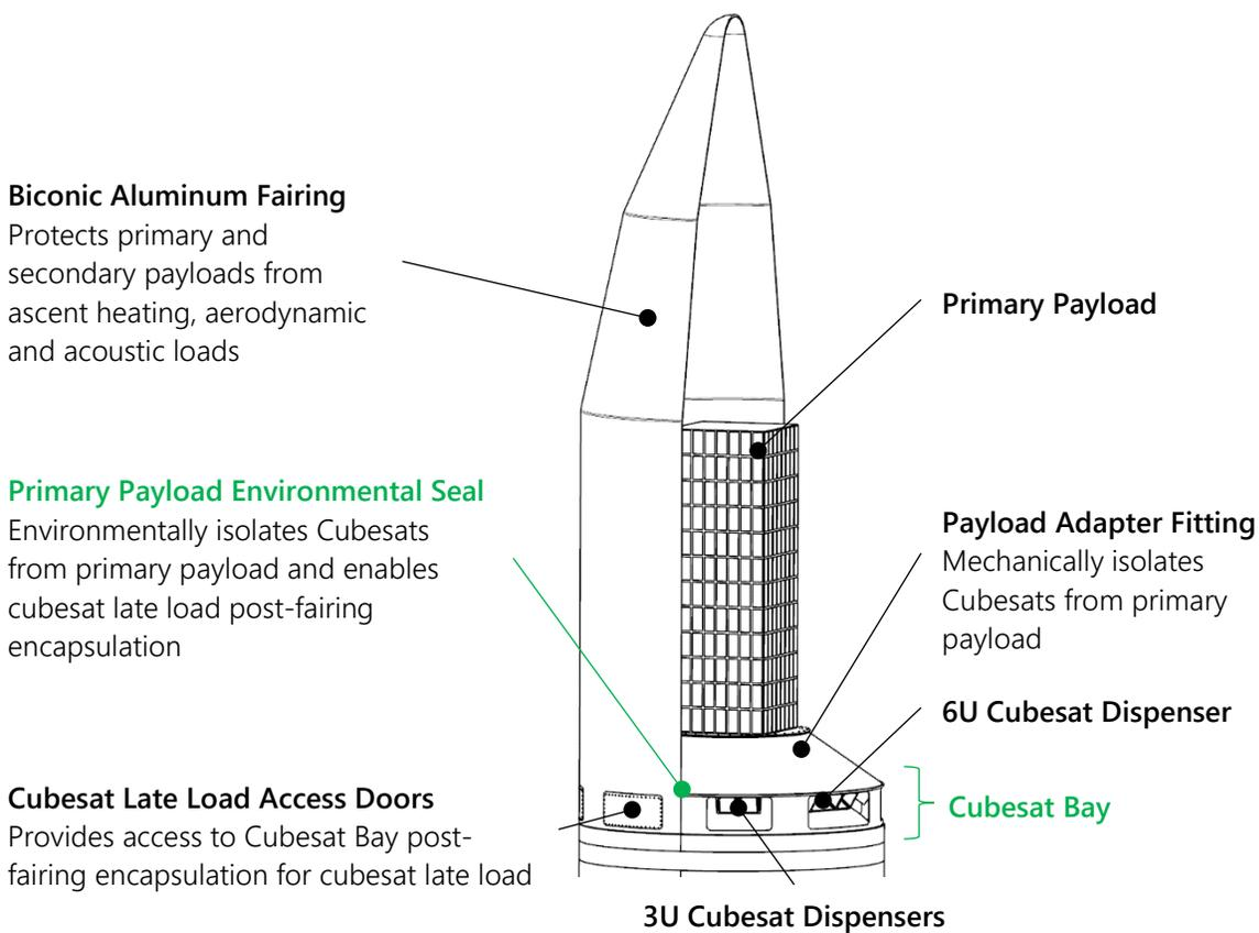
Figure 8: Payload Fairing with Cubesat Bay
