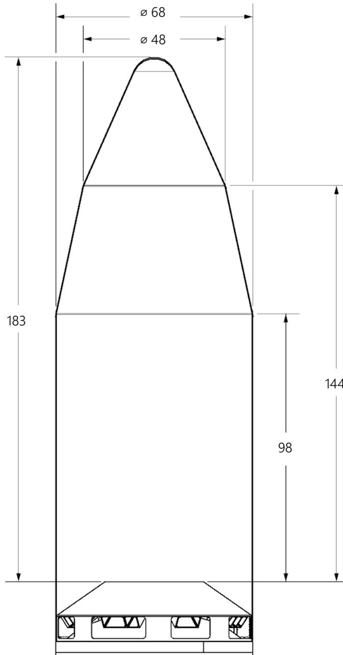
Figure 7: RS1 Payload Fairing Usable Volume Envelope (all values in inches)
