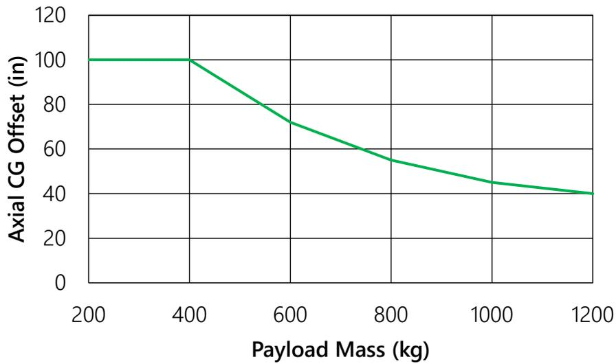
Figure 13: Primary Payload Axial Center of Gravity Limits
