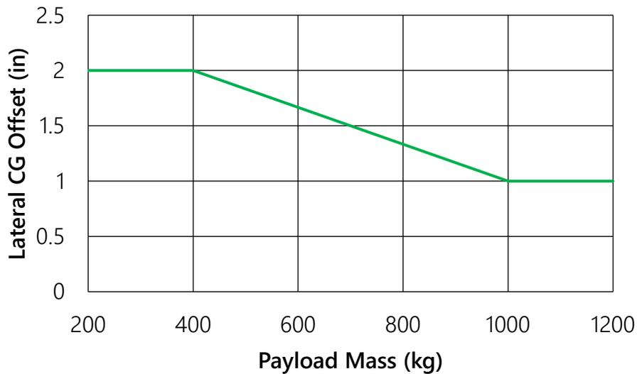
Figure 14: Primary Payload Lateral Center of Gravity Limits
