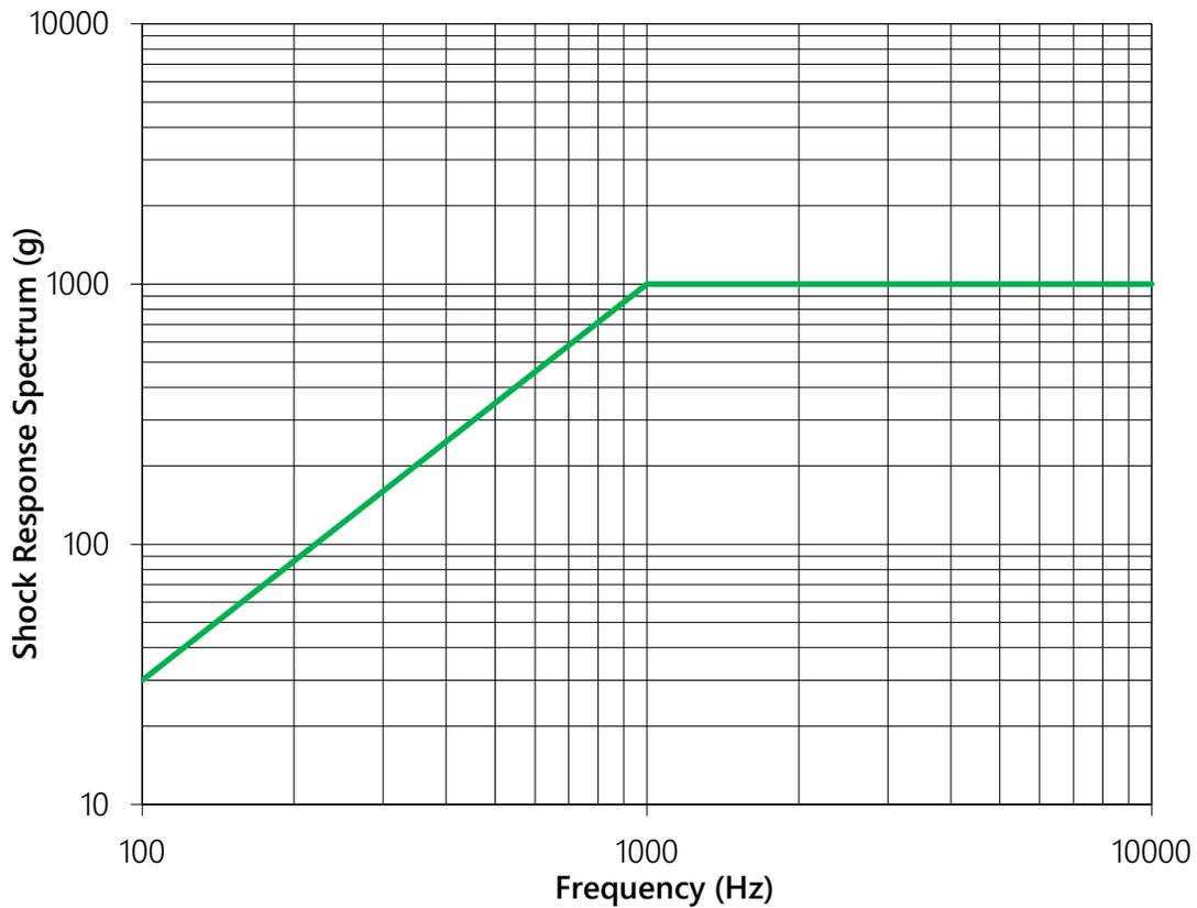
Figure 12: Approximate Shock Response for Payload Separation
