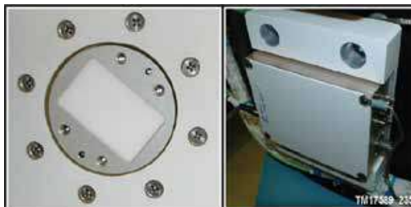
Figure 8.8-1. TDRSS 20W LCT2 Transmitter and Cavity Backed S-band Antenna
