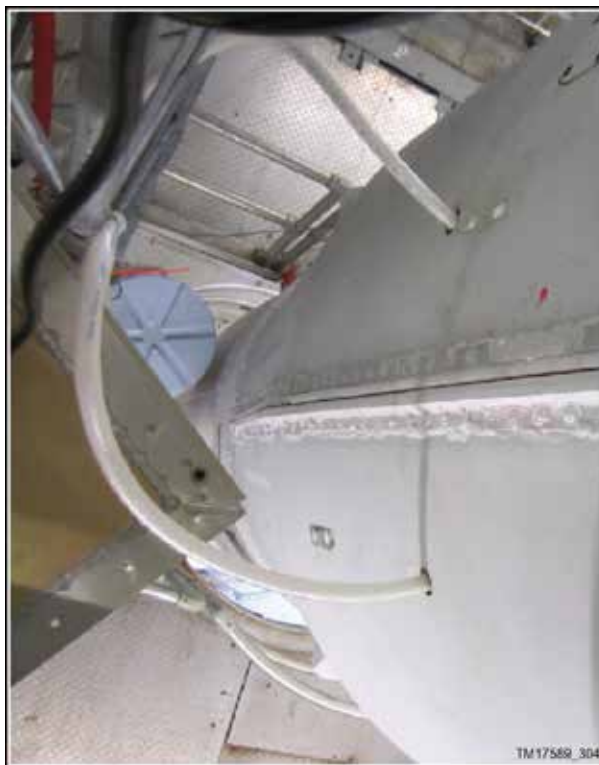
Figure 8.3-1. \text{GN}_2 Purge Interface To Minotaur Fairing (Flyaway at Liftoff)
