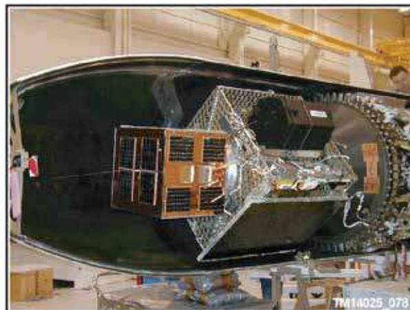
Figure 5.2.4.1.1-2. JAWSAT Multiple Payload Adapter Load Bearing Spacecraft
