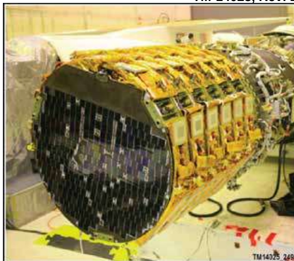
Figure 5.2.4.1.1-1. COSMIC Spacecraft Configuration Utilized the NGIS MicroStar Bus to Fly Six SVs
