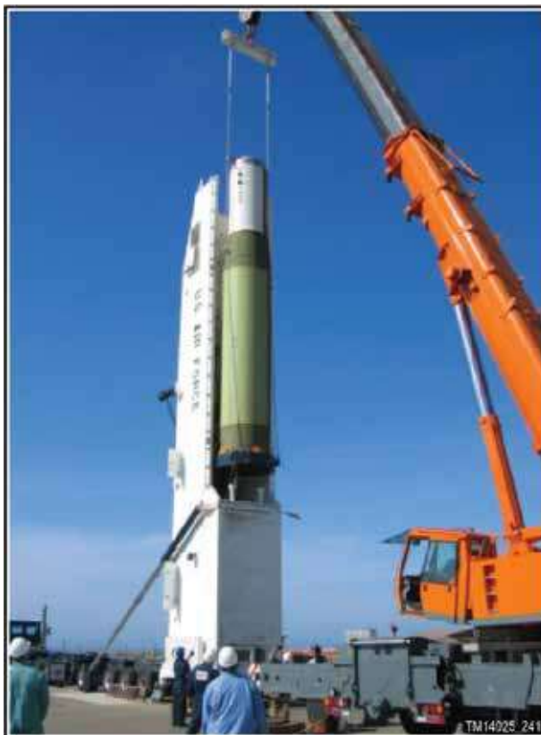
Figure 2.3.1-1. Minotaur I LSA Being Lifted out of Transporter Erector
