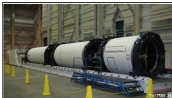
Figure 2.3.1-1. GFE Peacekeeper Stages 1, 2, and 3 Have an Extensive Flight History with over 50 Launches
