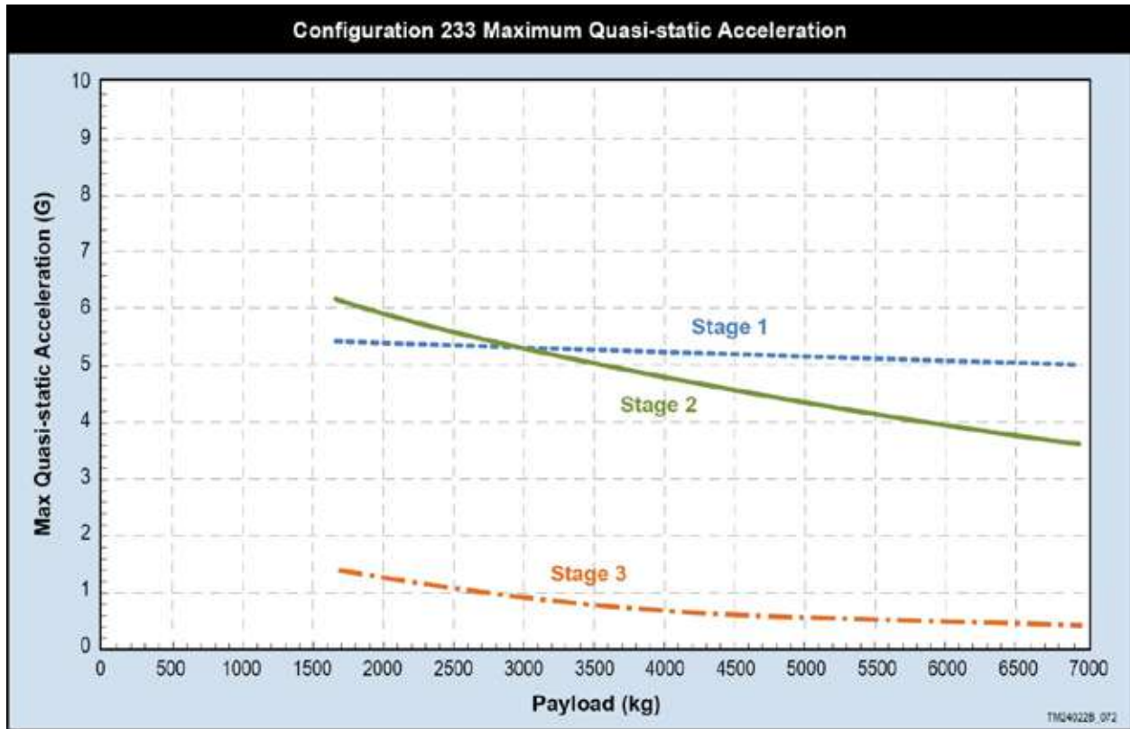
Figure 4.1.2-4. Antares 233 Nominal Payload Acceleration as a Function of Mass
