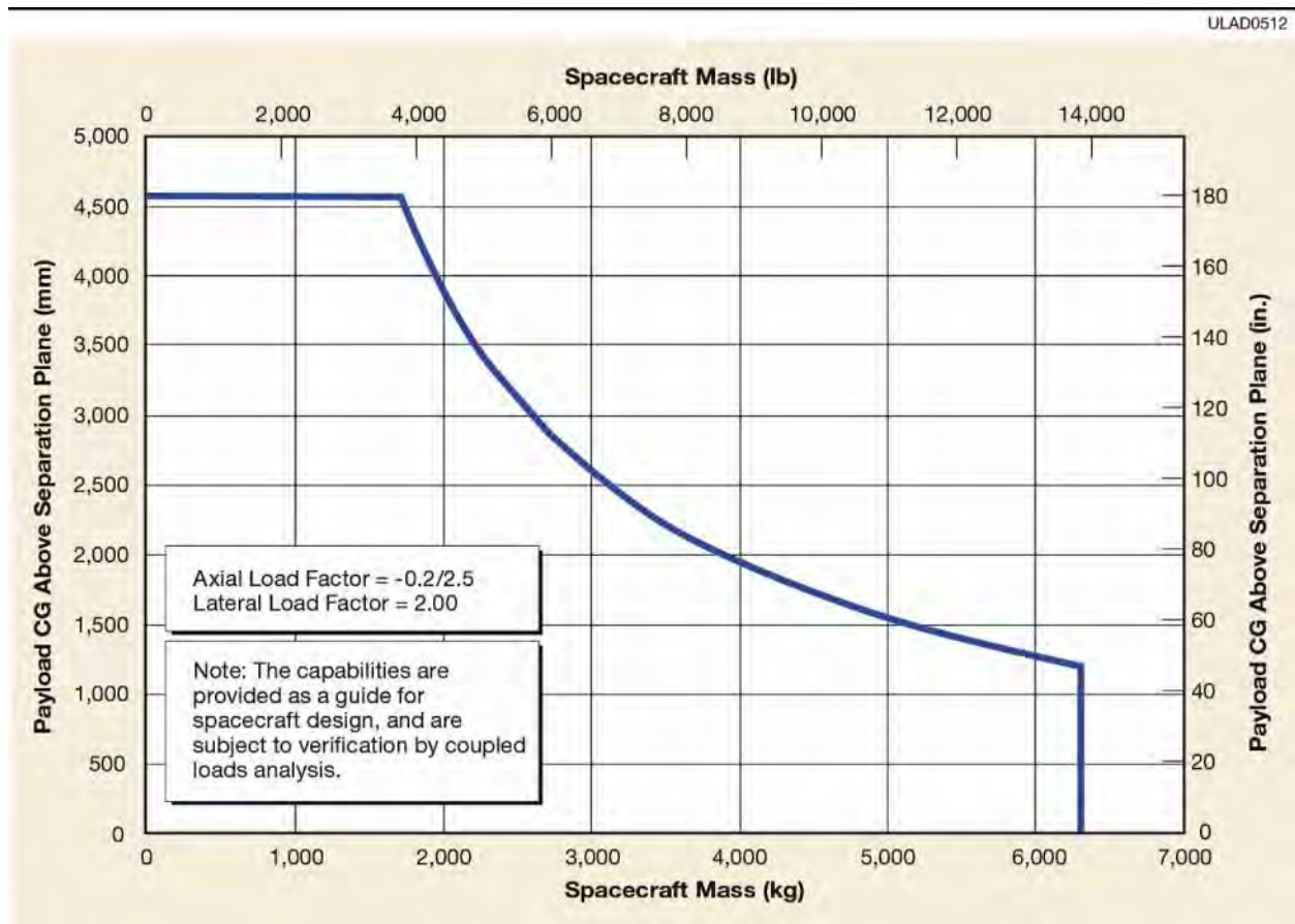
Figure 5-34. A937 PLA Structural Capability
