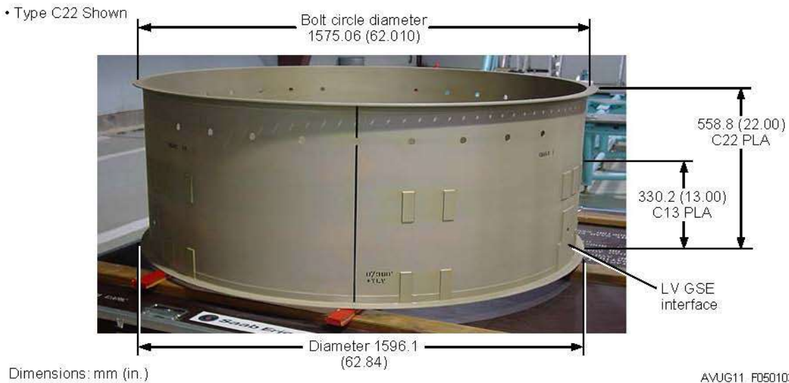
Figure 5.1.3-1: Atlas V Launch Vehicle Adapter Configuration
