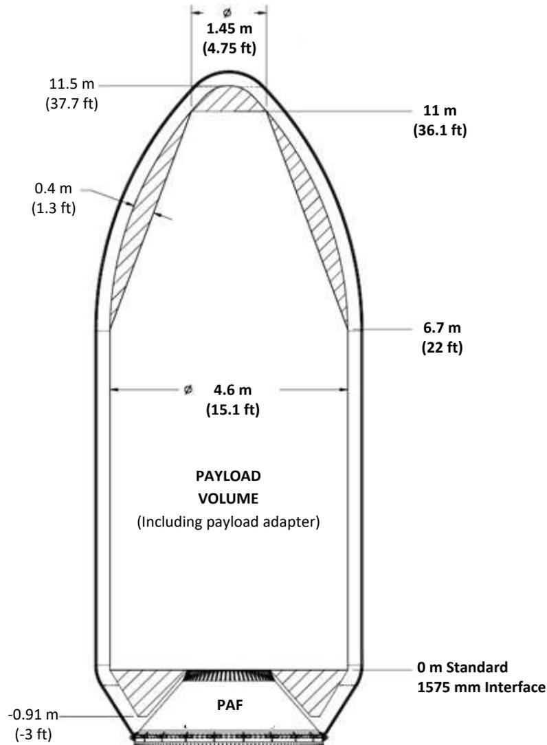
**Figure 5-1: Falcon fairing and payload dynamic envelope<sup>2</sup>, meters (feet)**
