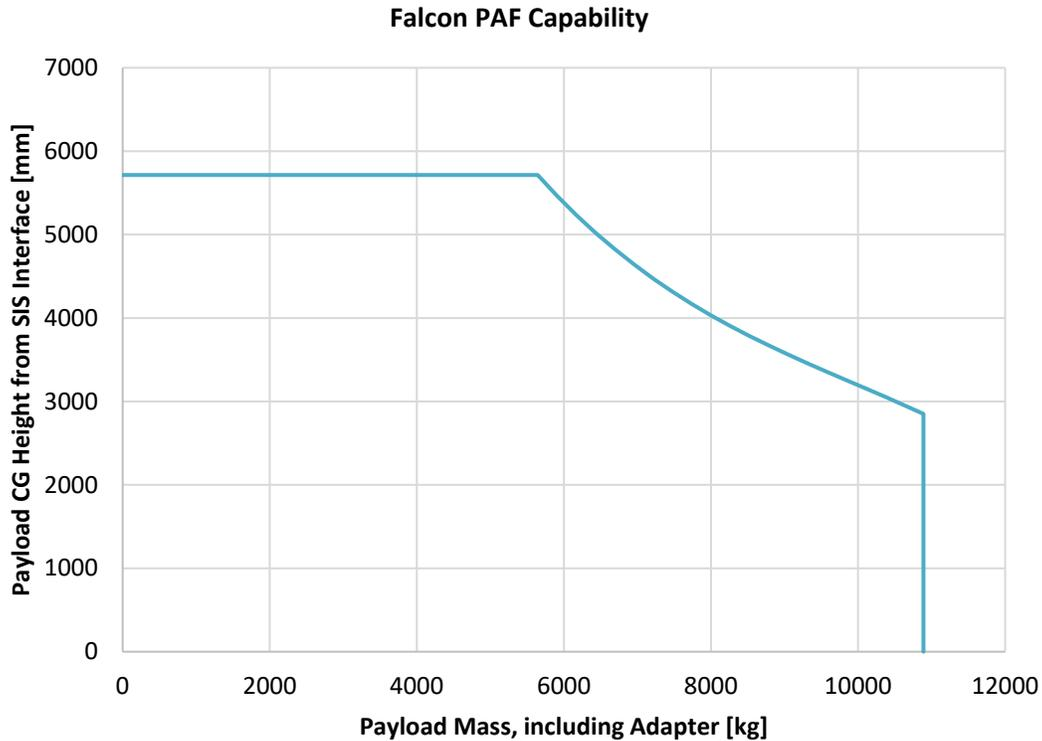
**Figure 3-2: Allowable center-of-gravity height above the 1575-mm plane**
