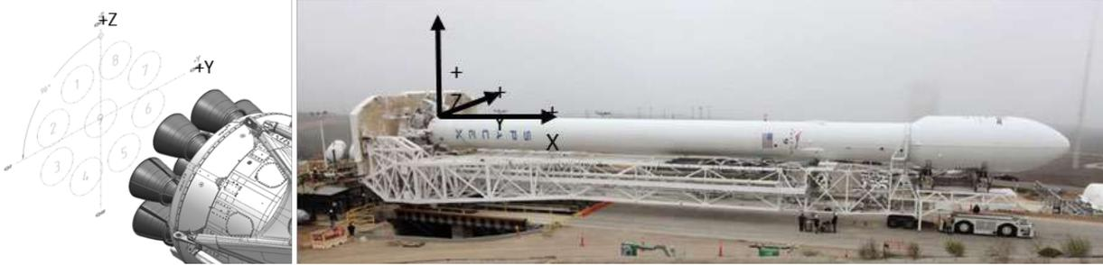
**Figure 2-4: Falcon vehicle coordinate frame**
