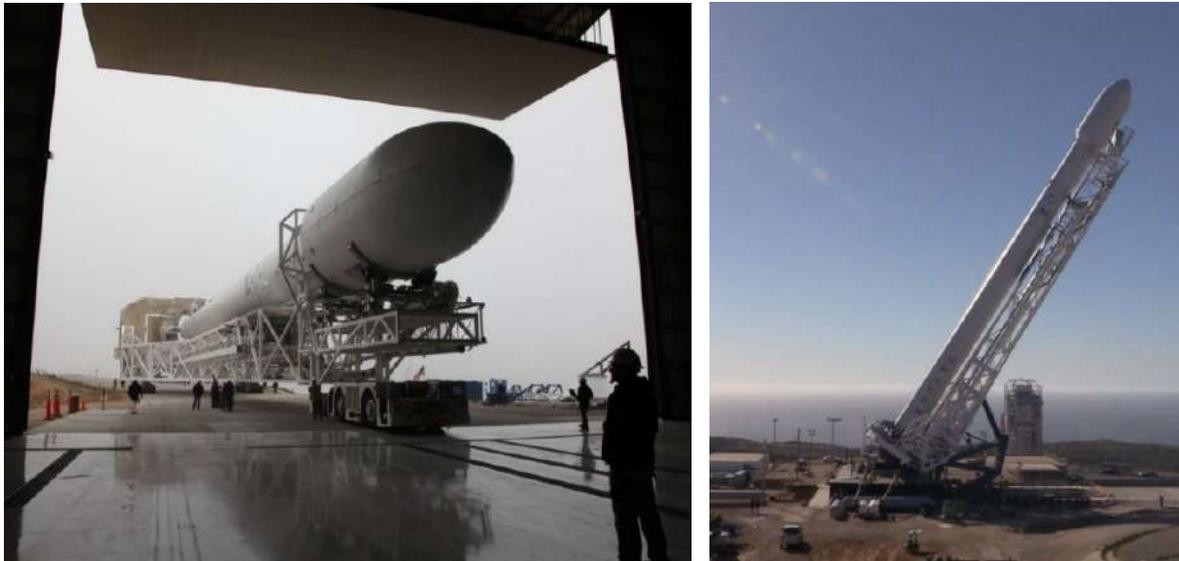
Figure 8-9: Launch vehicle rollout and erection
