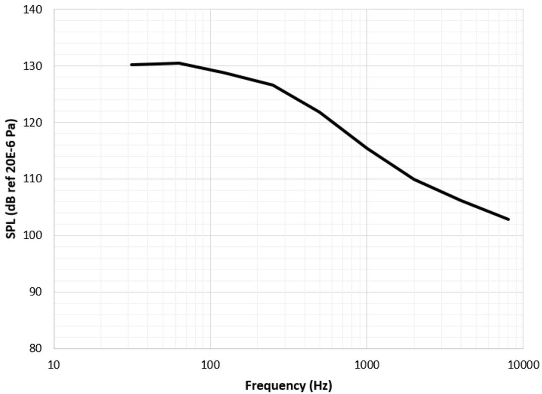
Figure 4-8: Falcon Heavy maximum predicted acoustic environment (P95/50), 60% fill-factor, 135.6 dB OASPL (full octave)
