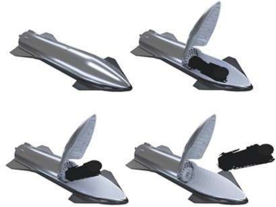
Figure 3: Starship payload deployment sequence
