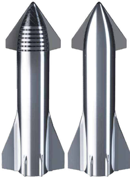
Figure 2: Starship crew (left) and uncrewed (right) configurations
