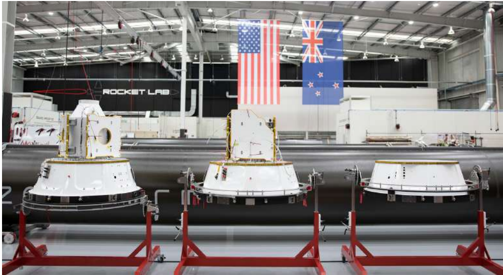
Figure 8 Rocket Lab's Kick Stages for three different missions
