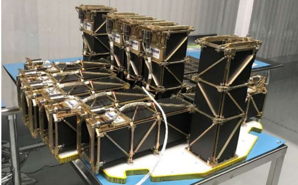
Figure 30 Rocket Lab payload plate, payload configuration for NASA ELaNa-19 mission
