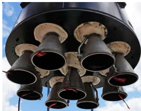
Figure 3 Rutherford Stage 1 Configuration
