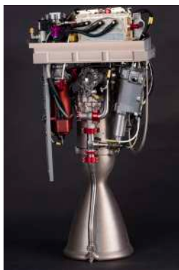
Figure 2 First Stage Rutherford Engine
