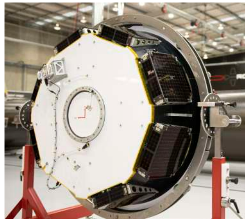
Figure 12 Photon LEO configuration (payload plate view)
