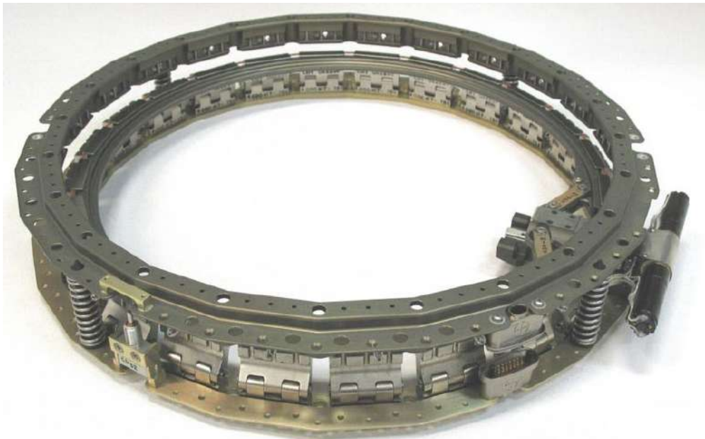
Figure 32 PSC Motorized Light Band (MLB) separation system
