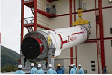
Assembling 1 st motor
