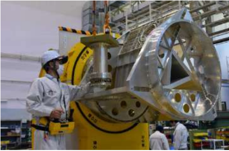
Multi-satellite mount structure
